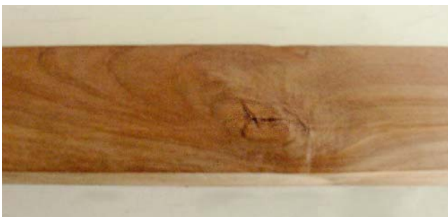
Fig. 10 Crack formation on the wood sample heat treated with dry gas
